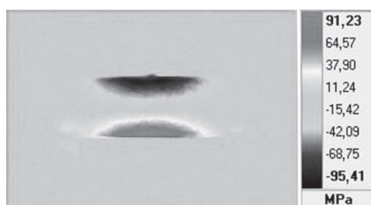
Figure 9 Distribution of principal stresses in the beam AISI 316TI specimen at 2 kN loading
