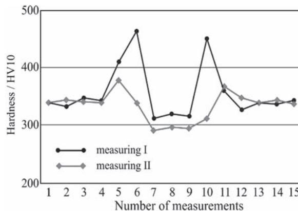
Figure 7 Dependence of hardness HV10 on measurement positions
