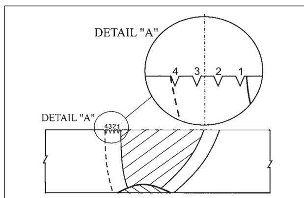
Figure 3 Position of V-notch in HAZ in relation to fusion line (V-notch position from the fusion line: 1 – 0,5 mm; 2 - 1,0 mm; 3 - 1,5 mm and 4 - 2,0 mm)
