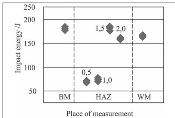
Figure 4 Results of testing the impact energy for mean value  $E_{ef} = 570$  J/mm
