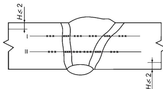
Figure 6 Positions for measuring of hardness in real welded joint
