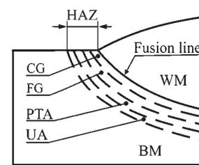
Figure 1 HAZ of single pass weld [1]
