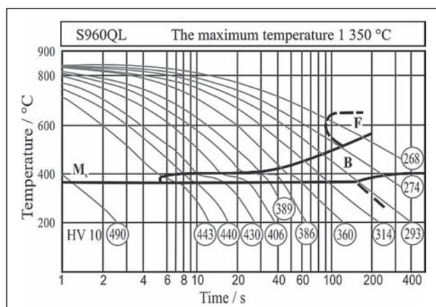
Figure 2 TTT diagram for S960QL steel [3]
