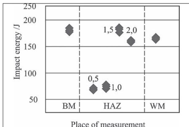
Figure 5 Results of testing the impact energy for mean value  $E_{ef} = 860$  J/mm
