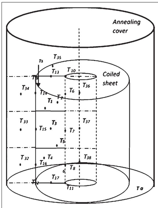
Figure 2 The scheme of thermocouple positions in coil space
