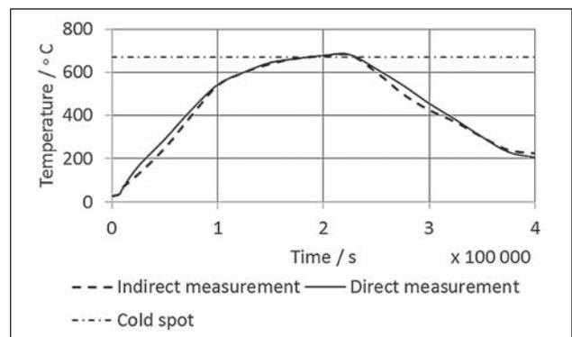
**Figure 5** Comparison of directly and indirectly measured inner temperature in point  $T_3$  for coiled sheet 2
