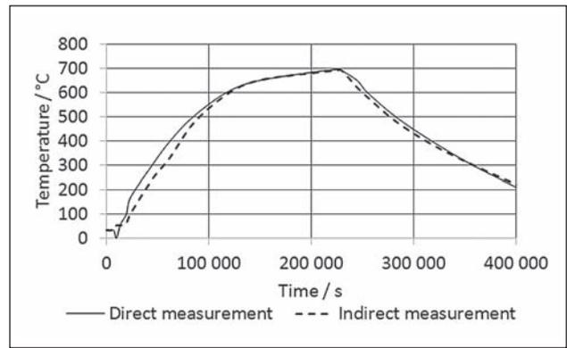
**Figure 4** Comparison of directly and indirectly measured inner temperature in point  $T_1$  for coiled sheet 2
