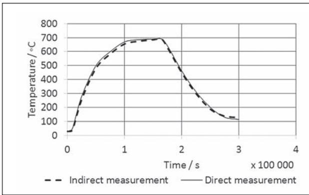
**Figure 3** Comparison of directly and indirectly measured temperature in point  $T_3$  for coiled sheet 1
