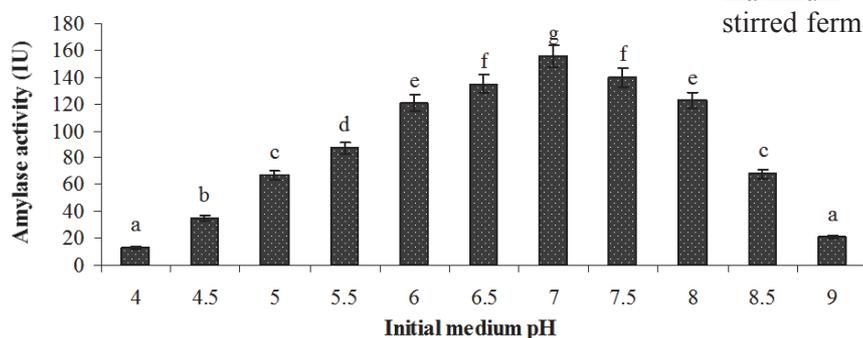
Fig. 2 – Effect of initial medium pH on amylase production in submerged fermentation
