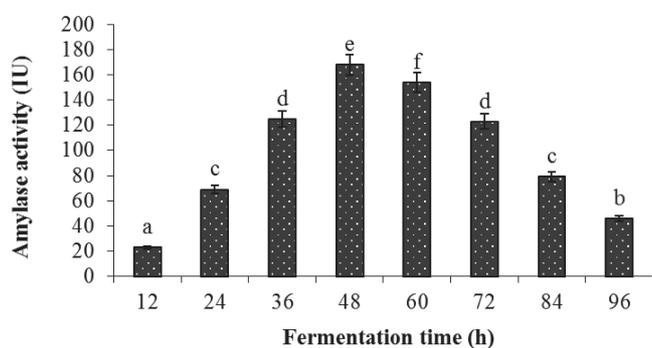
Fig. 1 – Effect of fermentation time on amylase production in submerged fermentation
