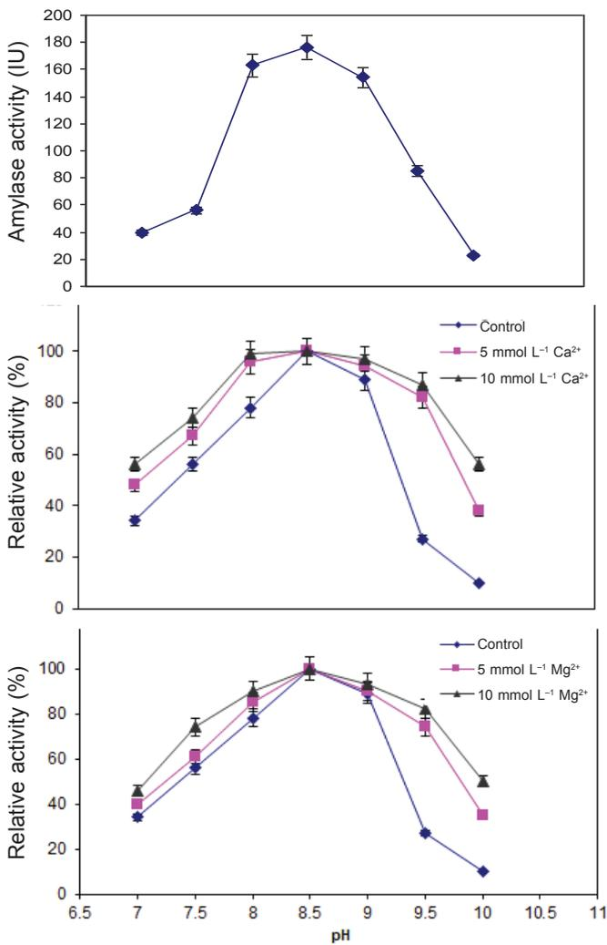
Fig. 9 – Effect of pH on activity and stability of amylase produced from *B. subtilis*
