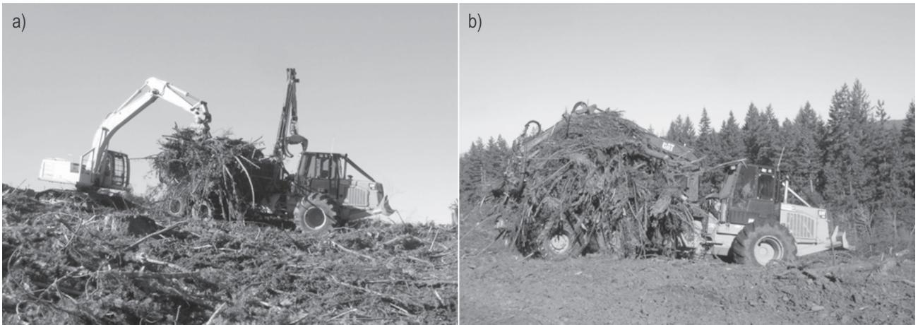
**Fig. 4** a) Forwarder being loaded by the excavator-base loader; b) Forwarder traveling to the landing
