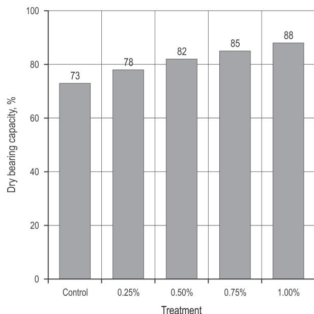
**Fig. 5** Variations of California bearing ratio (dry CBR) by increasing the percentage of CBR PLUS
