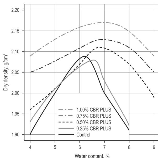
**Fig. 3** Dry density of materials treated by CBR PLUS in Proctor test
