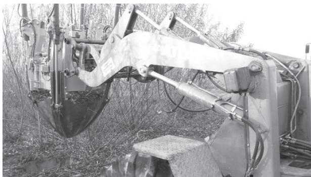
**Fig. 1** Root ball of an energy willow extracted using a head for transplanting large trees
