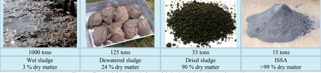
Figure 1 Characteristics of certain forms of sludge in relation to degree of processing
