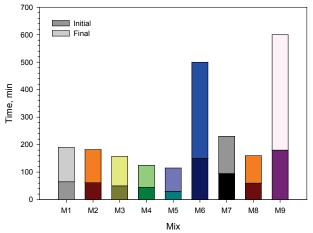
Figure 3 Influence of ISSA and additives on initial and final setting
