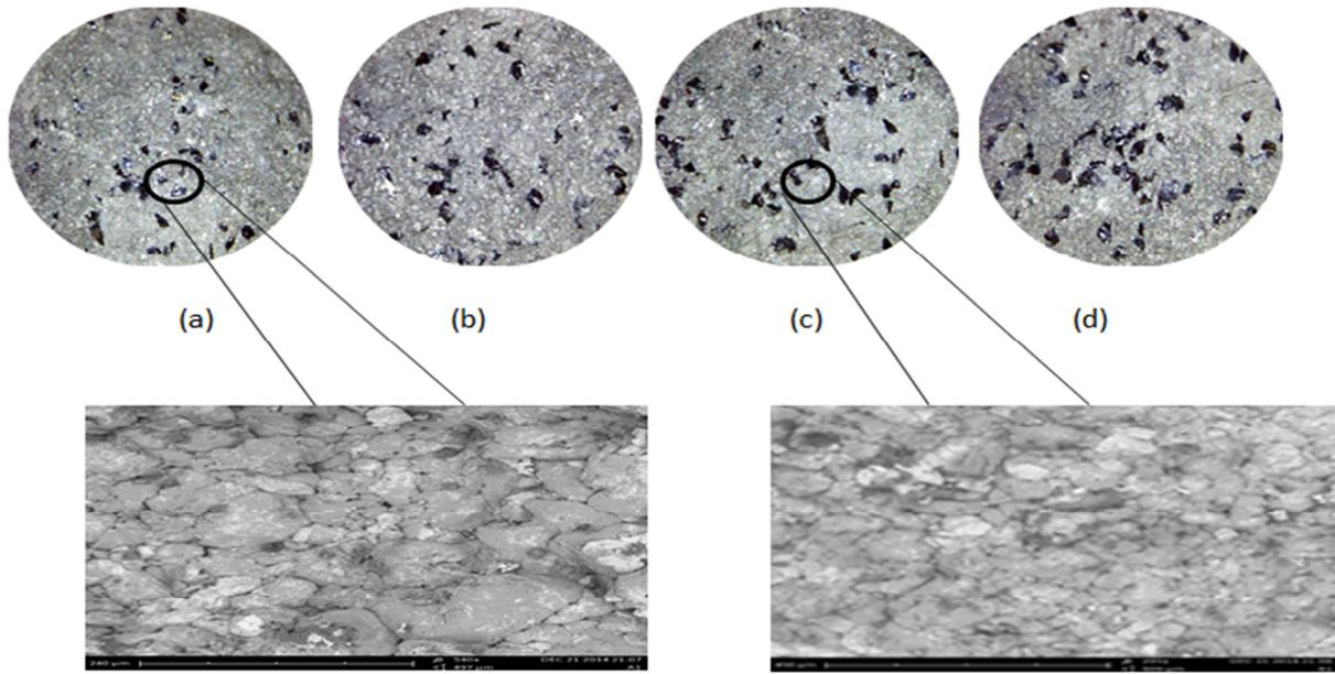
**Fig. 8** Microstructure of composites: (a) 0.5% vol. nano SiC, (b) 1.5% vol. nano SiC, (c) 3.5% vol. nano SiC and (d) 4.5% vol. nano SiC.
