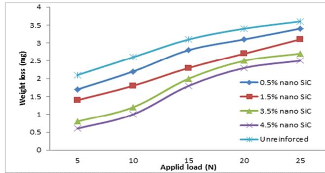
Fig. 4 Wear resistance at different applied loads
