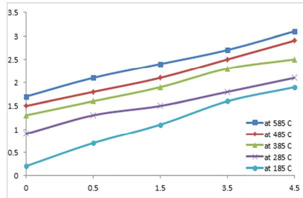
**Fig. 10** Variations in the porosity related to the vol. % of nano SiC content.
