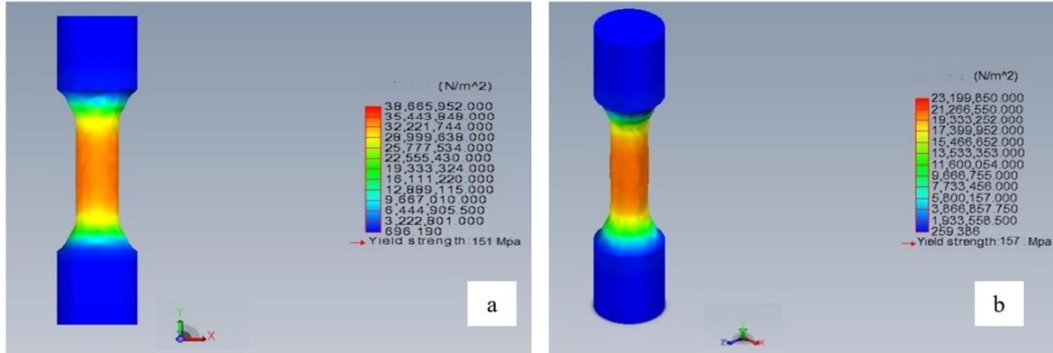
Fig. 13 Predicted yield strength of A356 reinforced with a) 1 vol. % nano SiC b) 2.5 vol. % nano SiC
