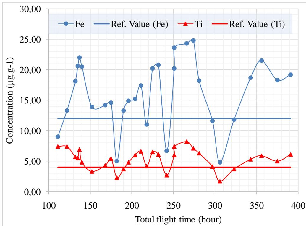
**Figure 2.** The course of changes in the concentration of Fe and Ti in over-all flight time
