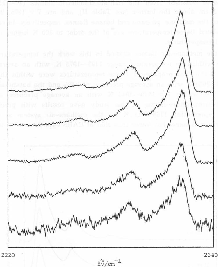
Figure 4. Stokes Raman spectra of nitrogen in butane-air flame,  $\Phi = 0.5$ . Axial distances 2.6 cm above burner orifice. Radial distance 0 mm from burner axis.
