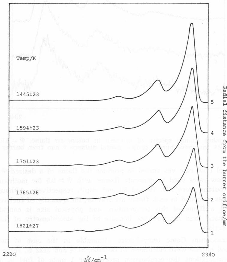
Figure 5. Stokes Raman spectra of nitrogen in propane-air flame,  $\Phi = 0.5$ . Radial distances 1–5 cm from burner axis at axial distance of 4 cm above burner orifice.
