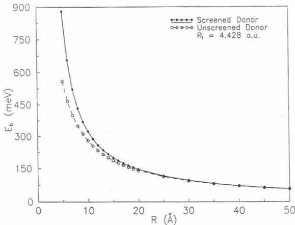
Figure 1. Binding energies (in meV) of screened and unscreened donors in a GaAs/Ga<sub>1-x</sub>Al<sub>x</sub>As QD of radius  $R$  (in Å).
