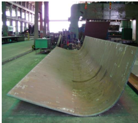
Fig. 5 Basic forming of amidships bilge plate
