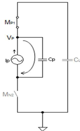
Fig. 7. Equivalent Circuit of Mode III Operation
