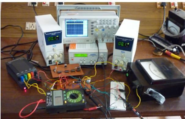
Fig. 18. Experimental setup of MOSFET Bridge AC to DC converter with switch control
