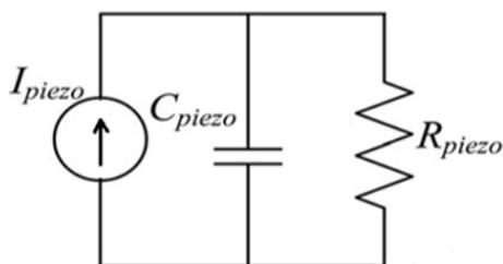
Fig. 2. Equivalent Circuit of a Piezoelectric Crystal
