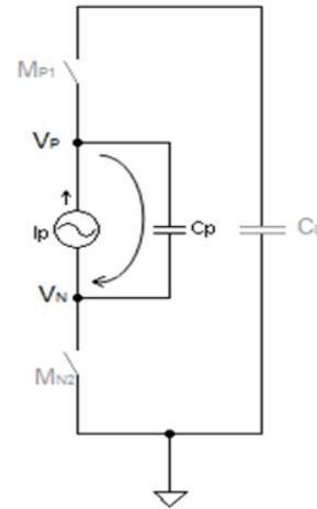
Fig. 5. Equivalent Circuit of Mode I Operation
