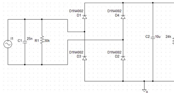
Fig. 8. Diode Bridge AC to DC converter
