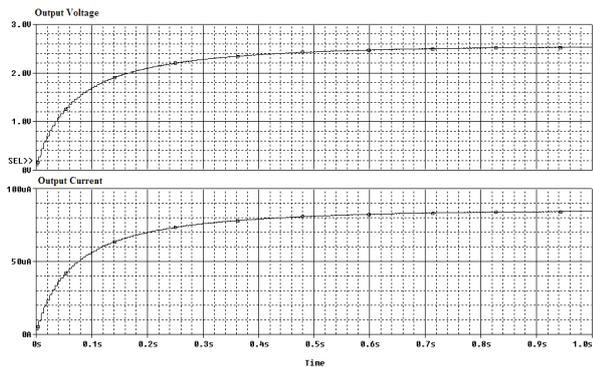
Fig. 16. Output Voltage and Current Waveforms of MOSFET Bridge AC to DC converter with Switch Control
