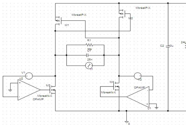
Fig. 11. MOSFET bridge AC to DC converter
