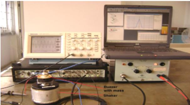
Fig. 17. Electromagnetic shaker and Piezo electric energy harvester
