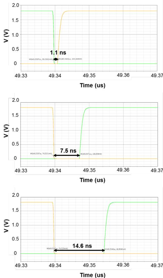
Fig. 7. Generated dead times using capacitance variation of the RC filter: (upper) 49.9 fF, (middle) 500 fF, and (lower) 1000 fF.
