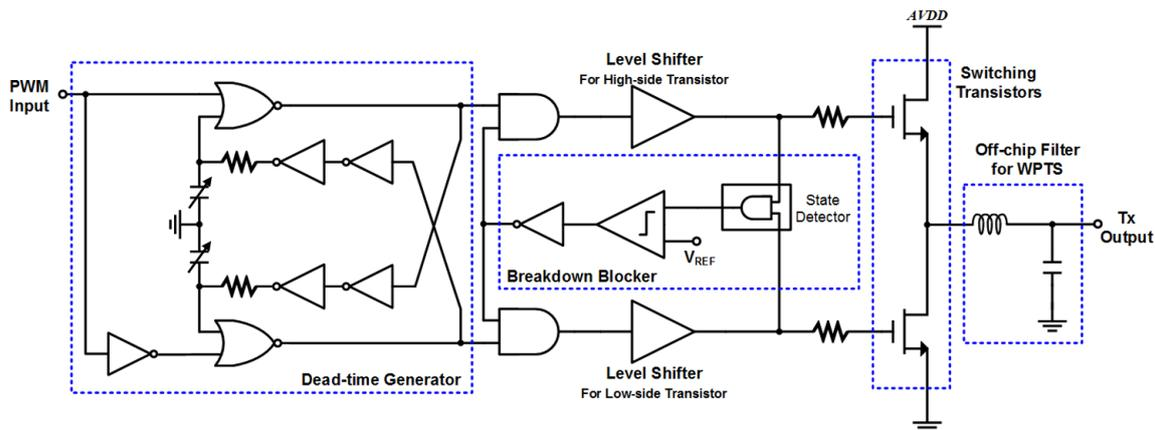
Fig. 2. Block diagram of the gate driver integrated circuit and the half-bridge power amplifier for the tightly-coupled wireless power transfer system (WPTS).
