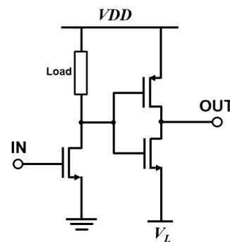
Fig. 4. Schematic diagram of the level shifter. The VDD is 5 V for the low-side switching transistor and AVDD for the high-side transistor. The V<sub>L</sub> is 0 V for the low-side and AVDD-5 V for the high-side.
