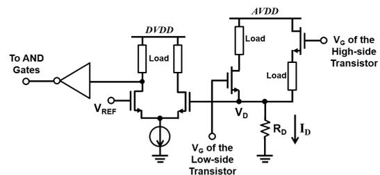
Fig. 5. Schematic diagrams of the breakdown blocker. The DVDD is the supply voltage of the digital logic circuits.
