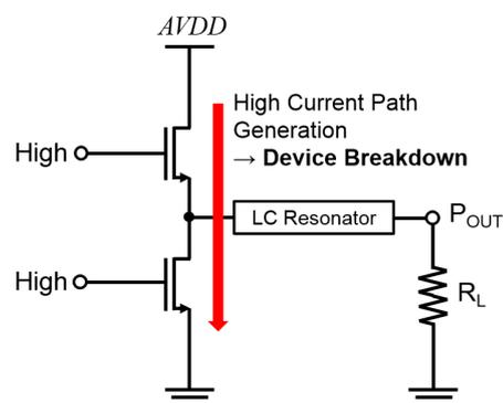
Fig. 1. Breakdown of Switching Transistors
