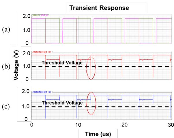
Fig. 10. Output voltage waveforms of the blocker depending on the value of the additional capacitance in the output node: (a) Input signals with overlapping time of 15 ns, (b) output of the breakdown blocker without the additional capacitor, and (c) output with the capacitor of 150 fF.
