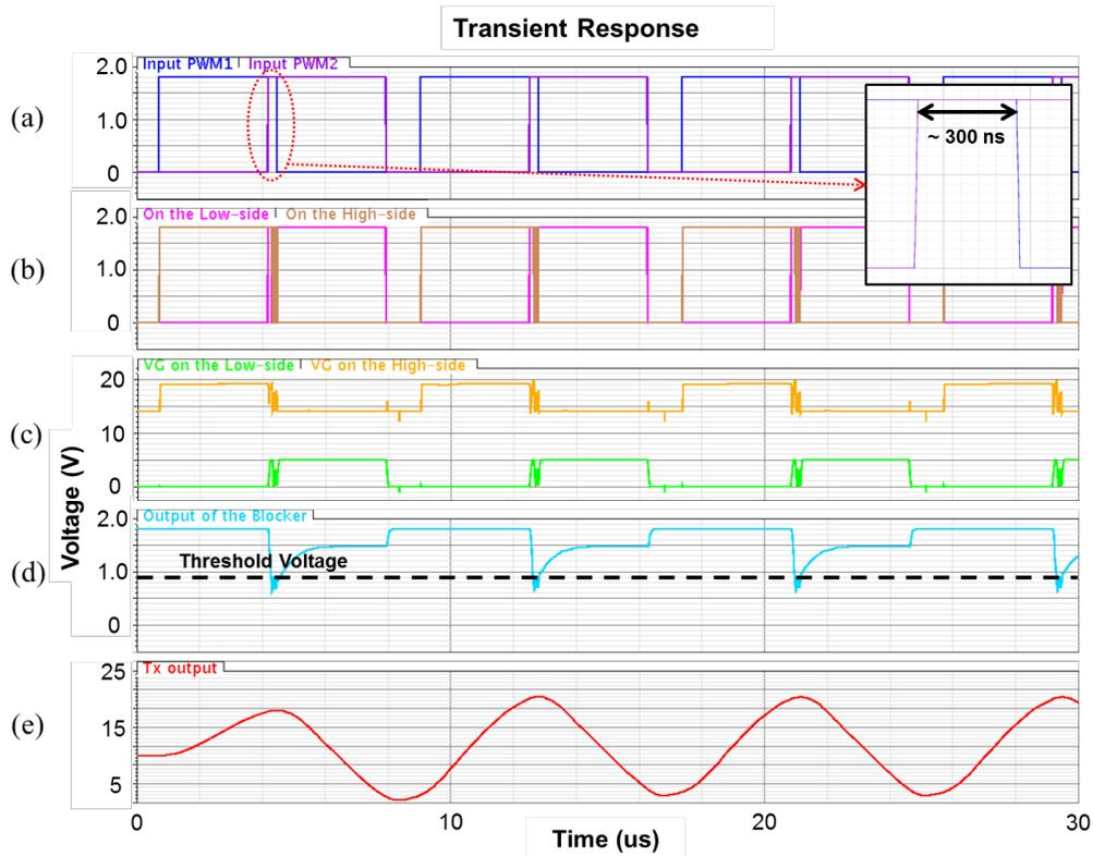
Fig. 9. Simulated voltage waveforms of the amplifier when 300 ns overlapping signals are connected to the output nodes of the dead-time generator: (a) Input overlapping signals, (b) inputs of the level shifters, (c) gate signals of the switching transistors, (d) output of the breakdown blocker, and (e) output of the amplifier. Block-box inset: Detailed view of the input overlapping signals.
