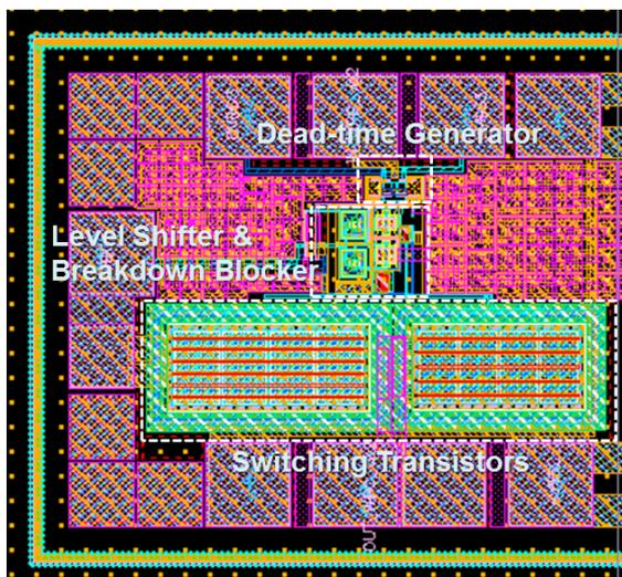
Fig. 3. Layout of the power amplifier with the proposed gate driver IC using TowerJazz's 0.18 μm BCD process.
