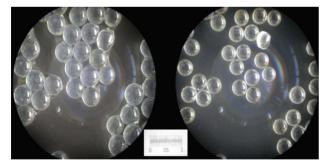
Fig. 6 – Ion exchanger particles during and after drying
