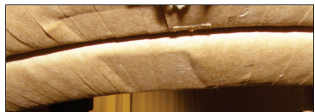
Figure 6 Squeezing of paper insulation
