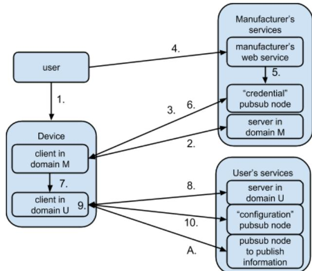
Fig. 7. Example of using pubsub for device configuration.
