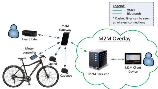
Fig. 8. Experimental M2M communication overlay based on XMPP.
