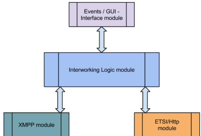
Fig. 9. The main functional modules and their relationships within the Interworking Proxy implementation.
