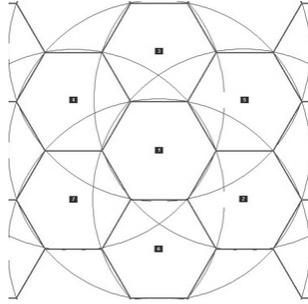
Fig. 9. Hexagonal Cells satisfy with 1.5 cell radius coverage
