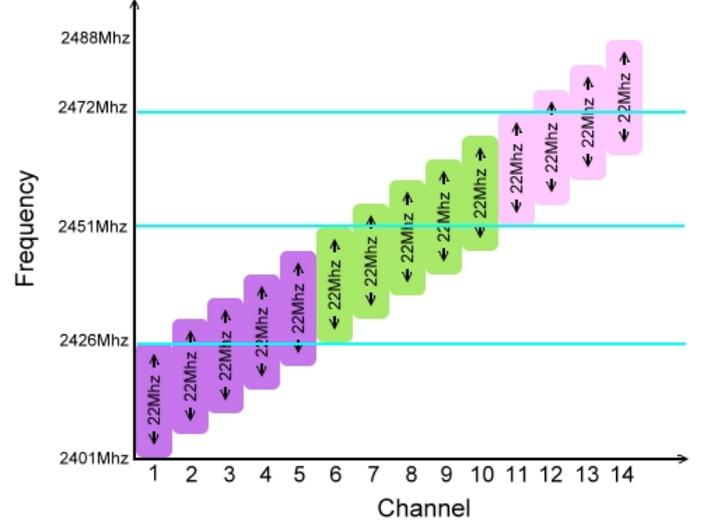
Fig. 11. IEEE 802.11b/g Frequency Spectrum to Channel Number
