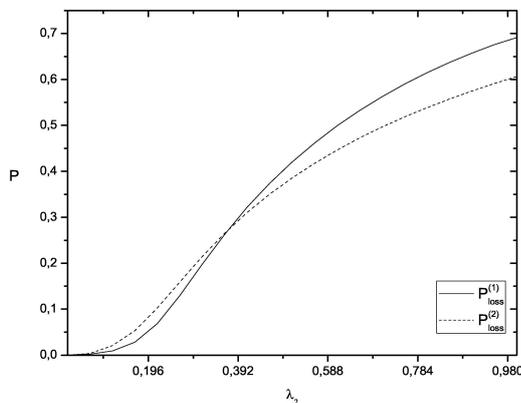
Fig. 4. Dependence of the loss probabilities  $P_{loss}^{(1)}$ ,  $P_{loss}^{(2)}$  on the intensity  $\lambda_2$  of priority packets
