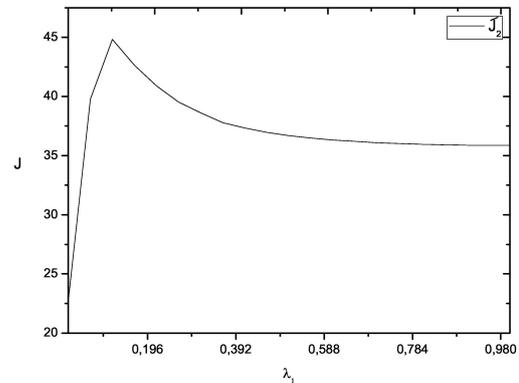
Fig. 3. Dependence of the jitter  $\tilde{J}_2$  of priority packets on the average intensity  $\lambda_1$  of non-priority packets
