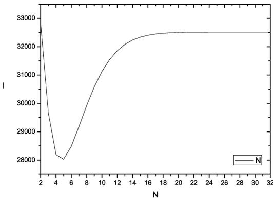
Fig. 10. Dependence of the economic criterion  $I_C$  on the available capacity  $N$  of the buffer for priority packets
