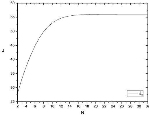
Fig. 9. Dependence of the jitter  $\tilde{J}_2$  on the available capacity  $N$  of the buffer for priority packets
