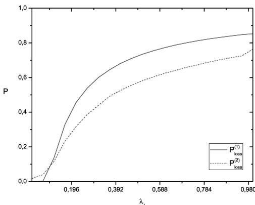
Fig. 2. Dependence of the loss probabilities  $P_{loss}^{(1)}$ ,  $P_{loss}^{(2)}$  on the average intensity  $\lambda_1$  of non-priority packets
