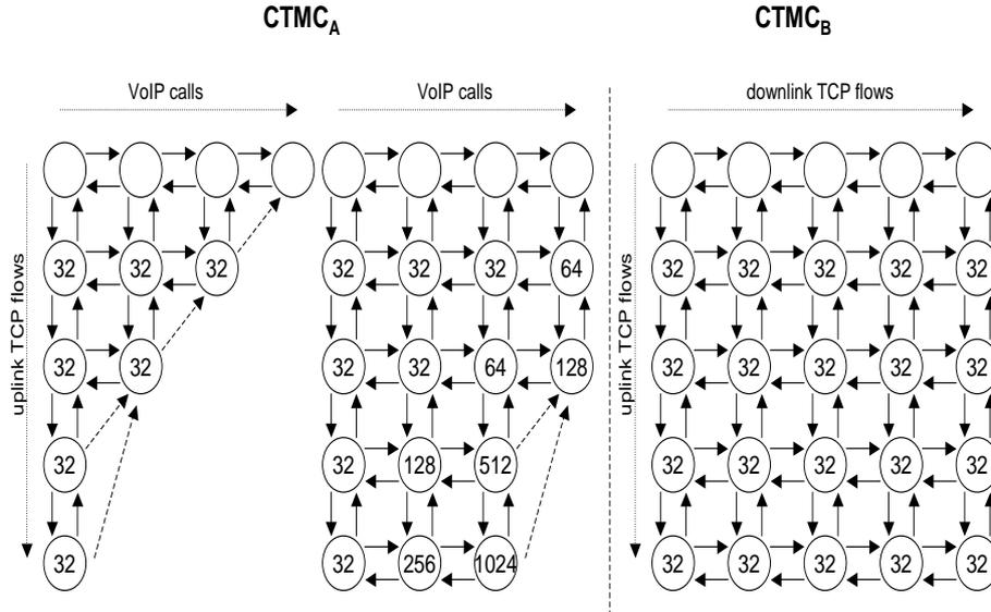
Fig. 3. CTMCs Example. Feasible states and  $CW_{min}$  values for uplink TCP flows. Dashed lines show the preemption transitions.
