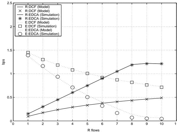
Fig. 2. Aggregate Throughput for elastic and rigid flows
