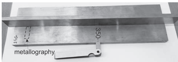
Figure 4 A view of friction surface on a plate made of high-chromium cast iron after tests in production conditions with marked area from which samples for metallographic tests were taken
