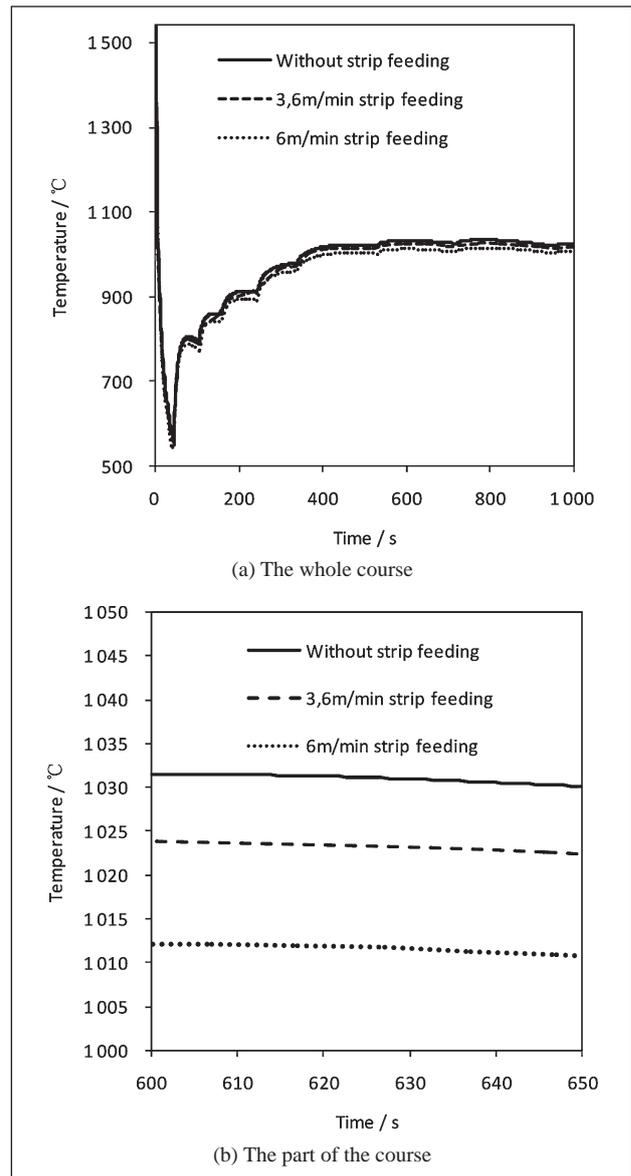
Figure 6 The comparison of temperature curves of different schemes in middle of narrow face
