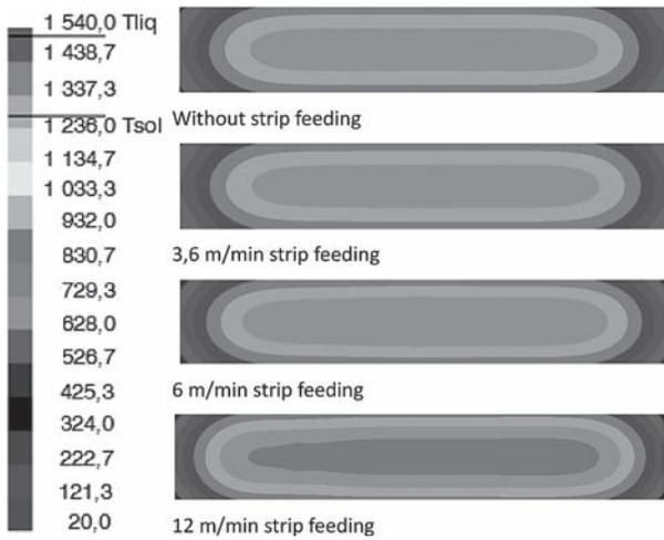
Figure 4 Comparison of temperature field in the end of solidification simulation
