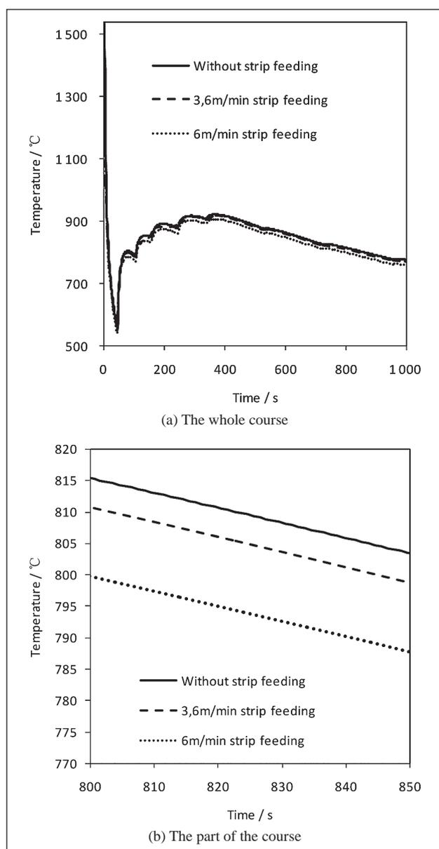
**Figure 7** The comparison of temperature curves of different schemes in middle of width face
