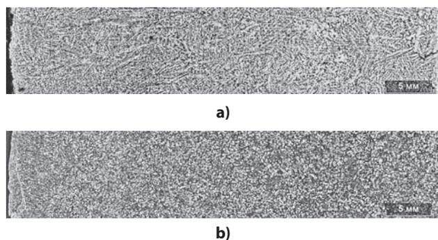
**Figure 2** Dendritic (a) and spherulitic (b) structure of cast metal: a) no conditioning agents added, b) with adding conditioning agent MM 0,2 kg/t
