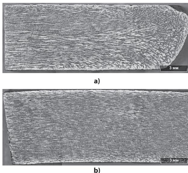
**Figure 4** Dendritic structure of the strip after controlled rolling: a) no modifiers added; b) modified by AKCeZh 2,3 kg/t
