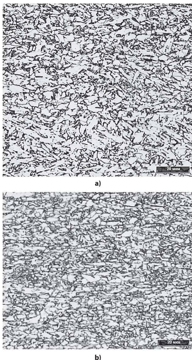
**Figure 3** Microstructure of the strip after controlled rolling: a) no modifiers added, b) modified by RZNTB 2,0 kg/t
