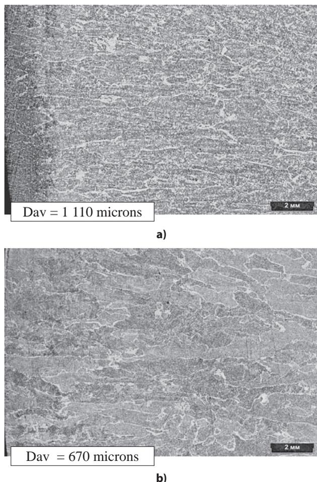
**Figure 1** Macrostructure of cast metal
