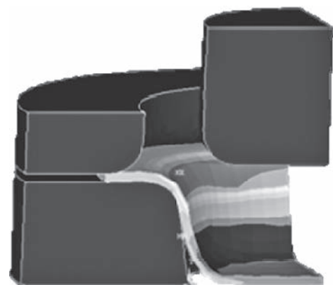
Figure 3 Disc deformation after 13 s of punch lowering.
