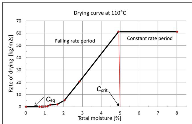
Figure 2. Drying curve during initial heating of the pressboard stack
