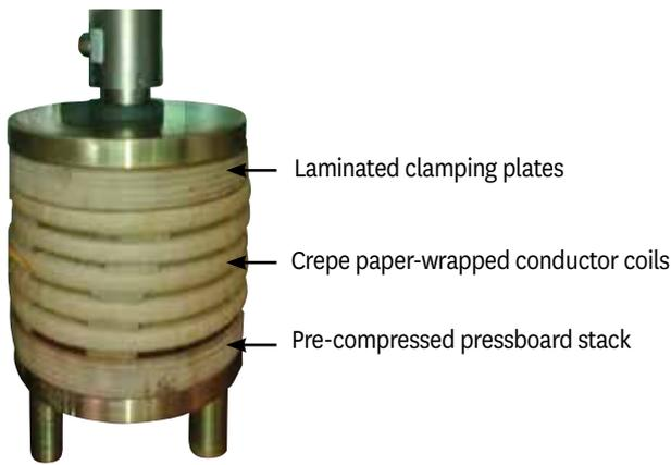
Figure 1. Lab scale model of typical core-coil assembly in a drying chamber
