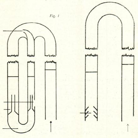
The bubbling of CO<sub>2</sub> through the mercury is sometimes so violent that mercury is sprayed out.
