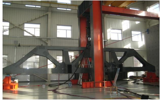
Figure 4. Experimental device of integral joint
