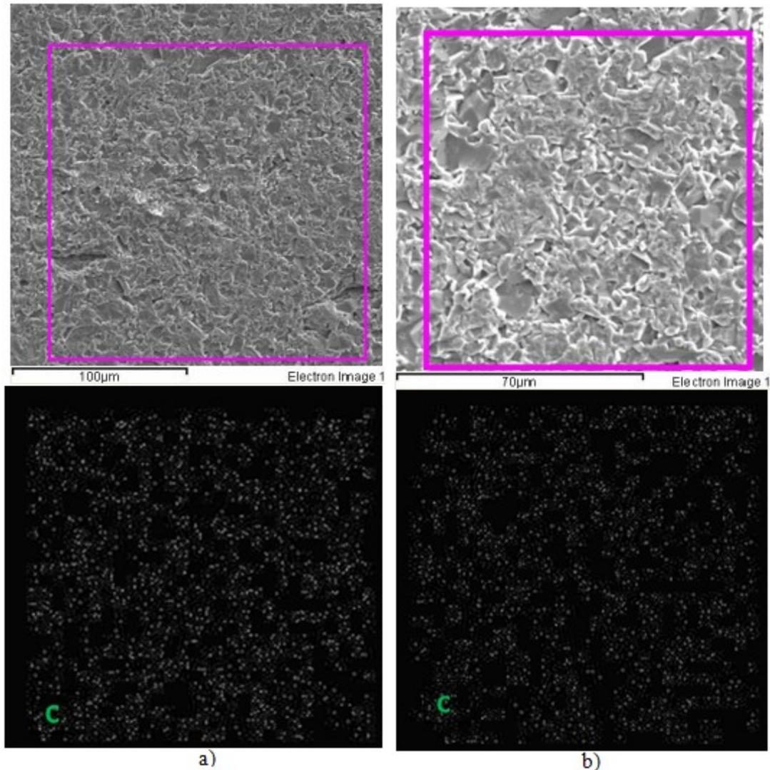
Figure 4. a) Distribution of carbon in the sample tested at magnification 500x
