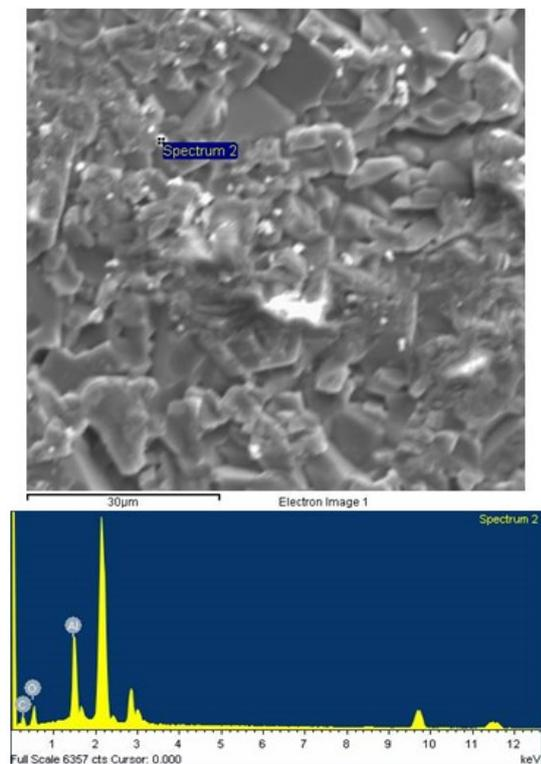
Figure 6. EDS spectrum of elements in the sample 2, magnification 2000x
