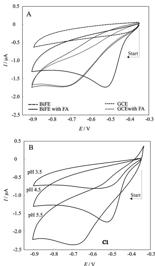
**Figure 2.** Cyclic voltammograms obtained at: (A) GCE and BiFE in  $0.1 \text{ mol L}^{-1}$  acetate buffer solution (pH 4.5) in absence and in presence of  $1.0 \times 10^{-4} \text{ mol L}^{-1}$  FA and (B) BiFE in acetate buffer solutions with different pH in presence of  $1.0 \times 10^{-4} \text{ mol L}^{-1}$  FA; (scan rate  $25 \text{ mV s}^{-1}$ ).
