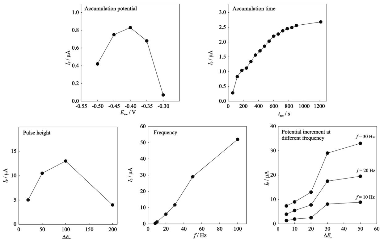
**Figure 4.** Effect of the electrochemical parameters on reduction peak current for SWCSV on BiFE in 0.1 mol L<sup>-1</sup> acetate buffer solution (pH 4.5) containing 1.0 μmol L<sup>-1</sup> FA. Optimizing time and potential accumulation was carried out with  $f = 10$  Hz,  $\Delta E_s = 20$  mV and  $\Delta E_p = 100$  mV.
