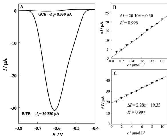
**Figure 5.** (A) SWCSVs with baseline correction, recorded at GCE and BiFE in 0.1 mol L<sup>-1</sup> acetate buffer solution (pH 4.5) in the presence of 5.0 μmol L<sup>-1</sup> FA; (B) calibration plot derived by subtracting background current from corresponding voltammograms for concentrations range 0.1–1.0 μmol L<sup>-1</sup>; (C) calibration plot derived by subtracting background current from corresponding voltammograms for concentration range 1.0–10.0 μmol L<sup>-1</sup>.
