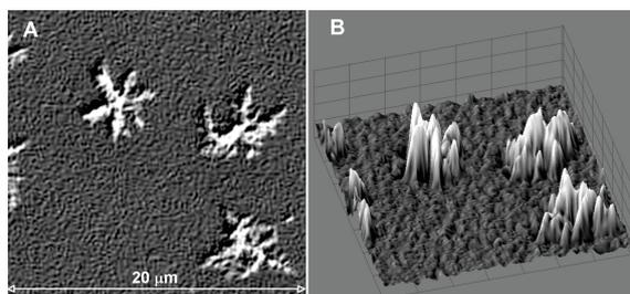
**Figure 1.** (A) part of SEM image at magnification 3000 $\times$  of the bismuth particles of film formed in  $0.1$  mol L<sup>-1</sup> acetate buffer solution (pH 4.5) containing  $1.0 \times 10^{-3}$  mol L<sup>-1</sup> Bi(III) and  $1.0 \times 10^{-3}$  mol L<sup>-1</sup> EDTA at  $-0.9$  V for 60 s; (B) cross-sectional view generated from SEM image.
