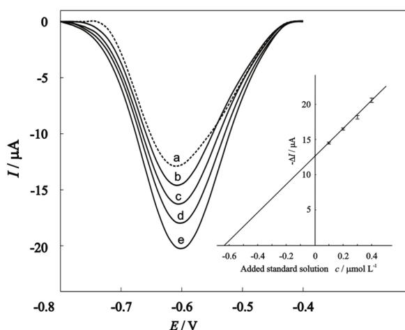
**Figure 6.** Analytical determination and recovery studies of FA in  $0.1 \text{ mol L}^{-1}$  acetate buffer solution (pH 4.5) at BiFE under optimized conditions for food supplement (Folacin) solution. Concentration of FA standard solution added: (a) supplement solution, (b)  $0.10 \mu\text{mol L}^{-1}$  (c)  $0.20 \mu\text{mol L}^{-1}$  (d)  $0.30 \mu\text{mol L}^{-1}$  (e)  $0.40 \mu\text{mol L}^{-1}$ .
