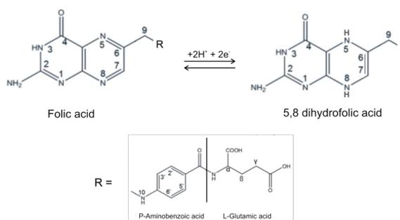
**Figure 3.** Reaction scheme for the electrochemical reduction of folic acid at pH 4.5.
