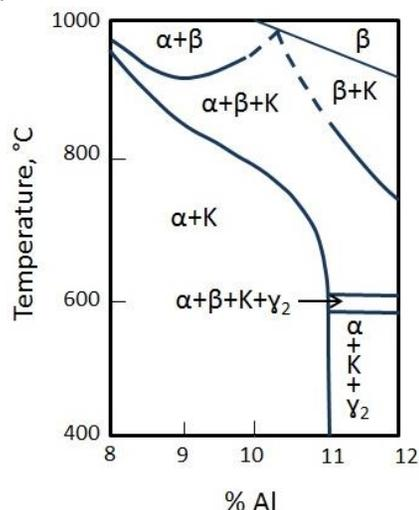
Figure 1 Vertical section through the Cu-Al-5%Ni-5%Fe phase diagram
