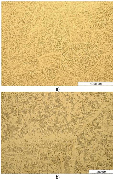
**Figure 2** Microstructural features of the as cast aluminum bronze samples showing a dendrite structure and different microconstituents: (a) Primary  $\alpha$ ; (b) Eutectoid  $\alpha+\gamma_2$  (100 $\times$  and 200 $\times$ )
