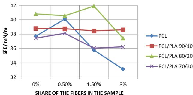
Figure 6 Surface free energy of samples
