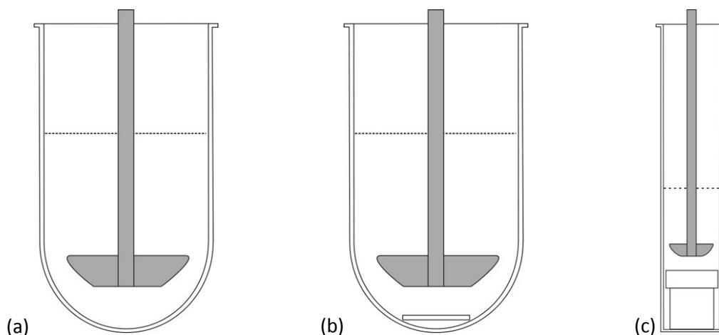
**Figure 2.** Schematic representation of the paddle apparatus (a), paddle over disc apparatus (b) and immersion cell in combination with the small-volume paddle apparatus (c). Reprinted from ref. [3] with permission of Elsevier.
