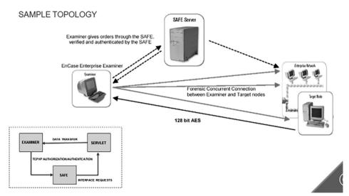
**Figure 2:** *EnCase* Enterprise implementation, picture is provided by courtesy of GuidanceSoftware
