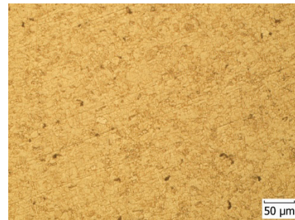
Figure 4 Microstructure of magnesium alloy AZ31
