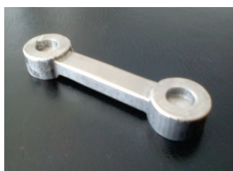
Figure 13 Final shape of Mg alloy drop forging
