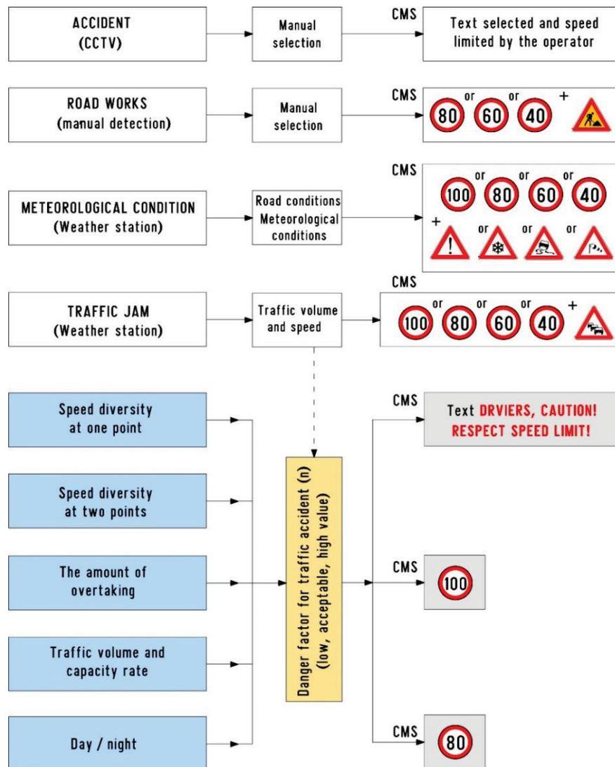
Figure 6 Algorithm for safety management, integrated with existing algorithms for traffic management on the test section (for one type of VMS and light text signs), (Source: prepared by authors)
