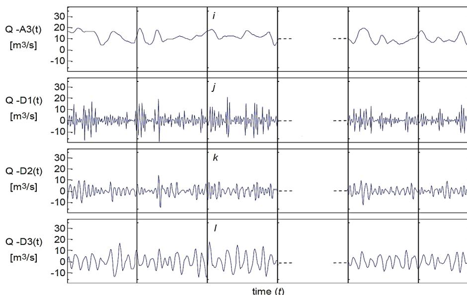
**Figure 4** Example of wavelet-aided approach to simulation of synthetic discharge time series. Series DWT components are divided on sections with similar properties and if *i*, *j*, *k* and *l* are not equal simultaneously then the reconstructed series presents newly simulated sequence (adapted from [34]).
