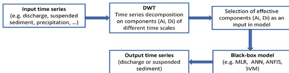
**Figure 3** Flow chart of methodology for discharge or suspended sediment forecasting with wavelet based hybrid black-box models
