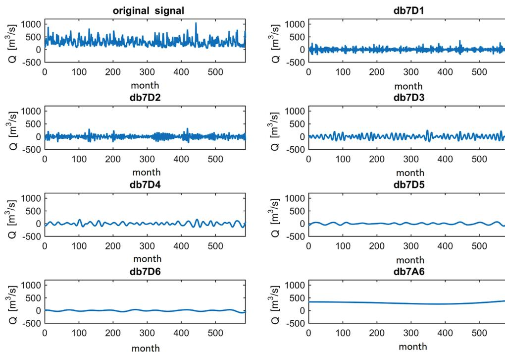
**Figure 2** Example of DWT decomposition of original monthly discharge time series on the six levels with db7 wavelet from GS Podused on the Sava River. Trend test of choice can be then done on reconstructed details ( $D_i$ ,  $i = 1, 2, \dots, 6$ ) of different time scales ( $2^i$  months,  $i = 1, 2, \dots, 6$ ) and remaining approximation ( $A_6$ ) and/or on different combinations of components [20].
