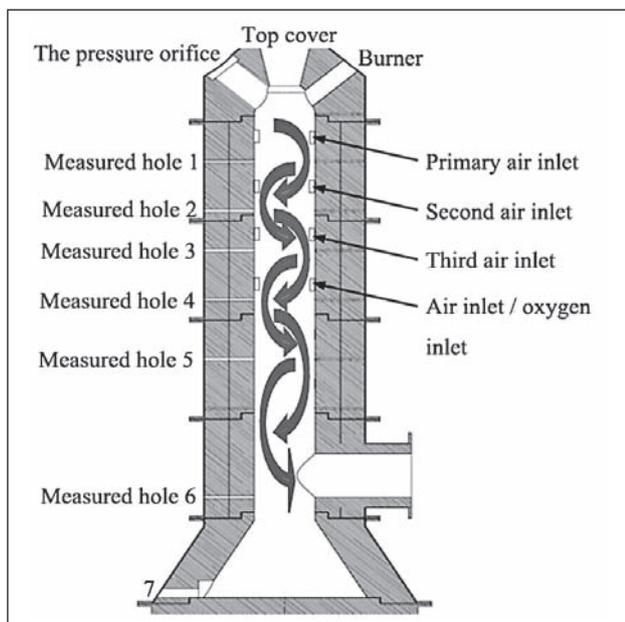
**Figure 1** Schematic diagram of the combustion system
