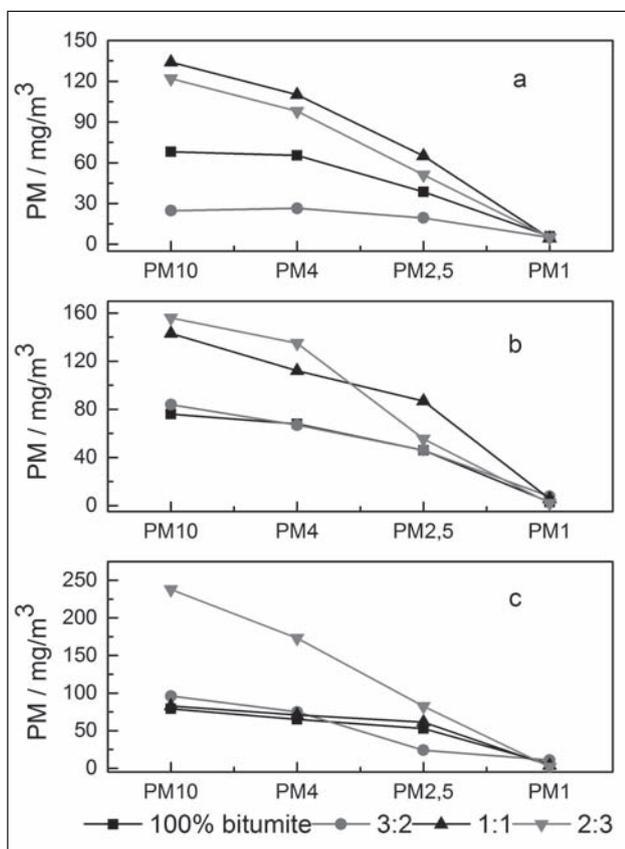
**Figure 4** Particulate matter concentrations under different coal ratios and fuel-staged ratio of 15:85 conditions. a) Air excess coefficient of 1,4. b) Air excess coefficient of 1,2. c) Air excess coefficient of 1,0.
