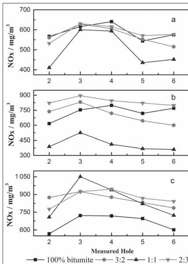
**Figure 2** Variation of the concentration of NO<sub>x</sub> for each measured hole under different coal ratios and fuel-staged is 15:85. a) Air excess coefficient of 1,4. b) Air excess coefficient of 1,2. c) Air excess coefficient of 1,0.
