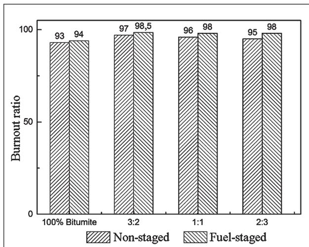
**Figure 3** Burnout ratios for the different coal ratios under non-staged and fuel-staged conditions
