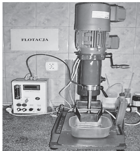
Figure 3 Laboratory flotation device used in the studies of flotation process
