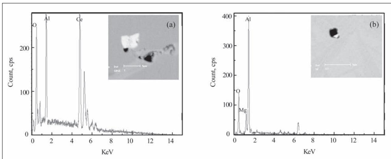
Figure 2 SEM images and EDS analysis results of typical inclusions
