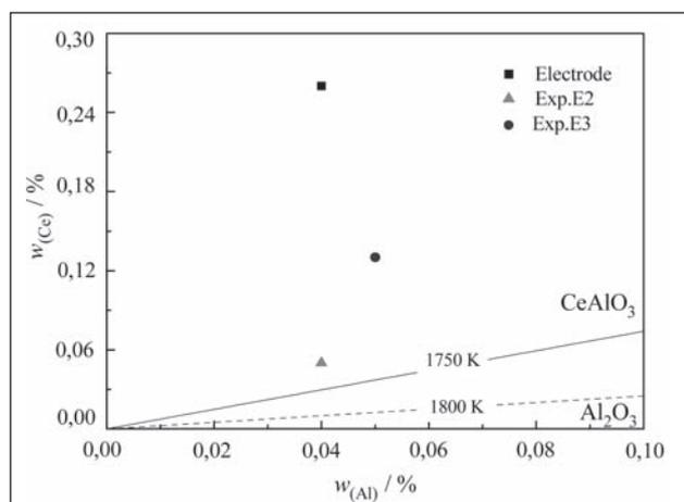
Figure 3 Diagrams of CeAlO<sub>3</sub>/Al<sub>2</sub>O<sub>3</sub> inclusions
