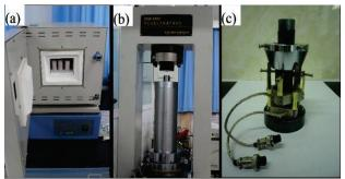
**Figure 1** Experimental equipment (a) FP-25 electric high temperature furnace and, (b) TAW-1000 electro-hydraulic servo controlled triaxial testing machine, (c) Axial and radial displacement transducers
