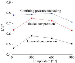
Figure 10 Relationship between  $U^e/U$  and treated temperature
