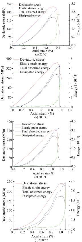
Figure 7 Energy evolution of granite after heat treatment under confining pressure unloading
