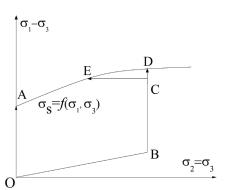
Figure 2 Sketch of three loading paths for granite samples
