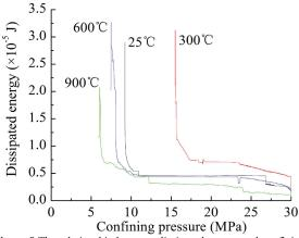
Figure 8 The relationship between dissipated energy and confining pressure of granite after high-temperature under confining pressure
