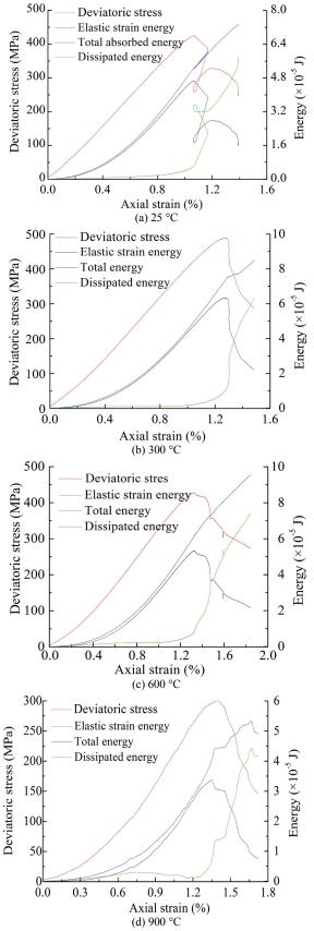
Figure 6 Energy evolution of granite after heat treatment under triaxial compression
