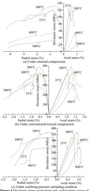
Figure 4 Deviatoric stress-axial strain and -radial strain curves of granite after high-temperature under three different loading paths
