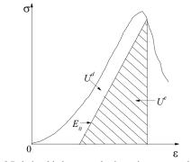
Figure 3 Relationship between elastic strain energy and dissipated energy of rock sample
