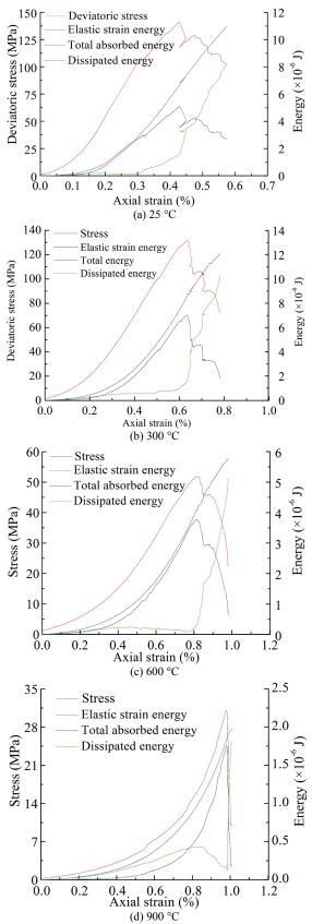
Figure 5 Energy evolution of granite after heat treatment under uniaxial compression
