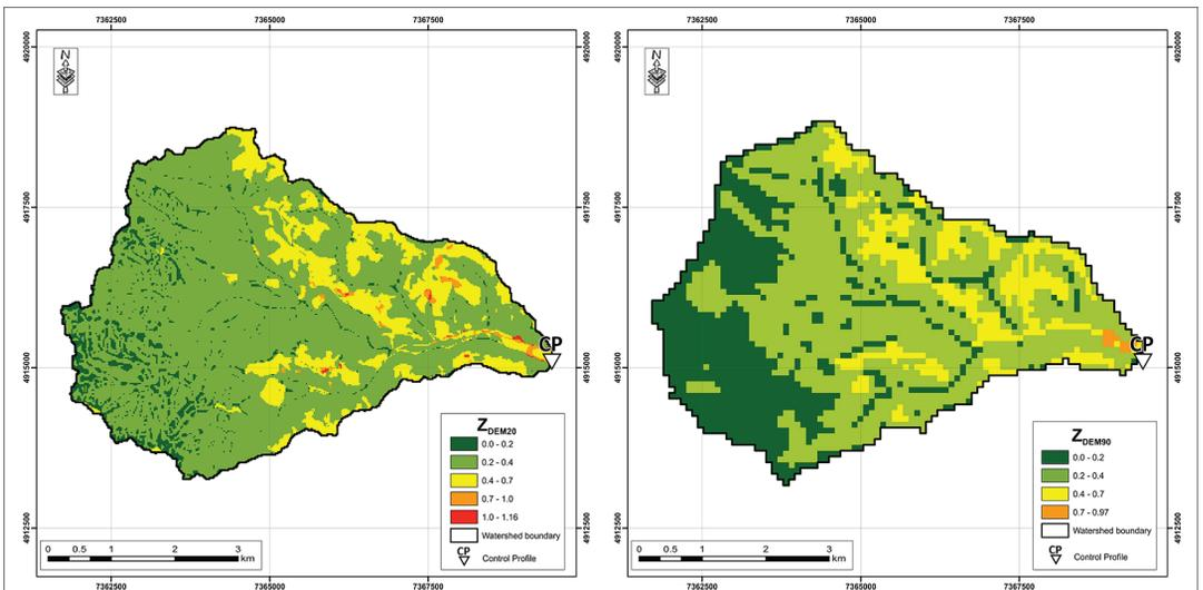
FIGURE 3. Spatial distribution of erosion coefficient Z (DEM<sub>20</sub> and DEM<sub>90</sub>)
