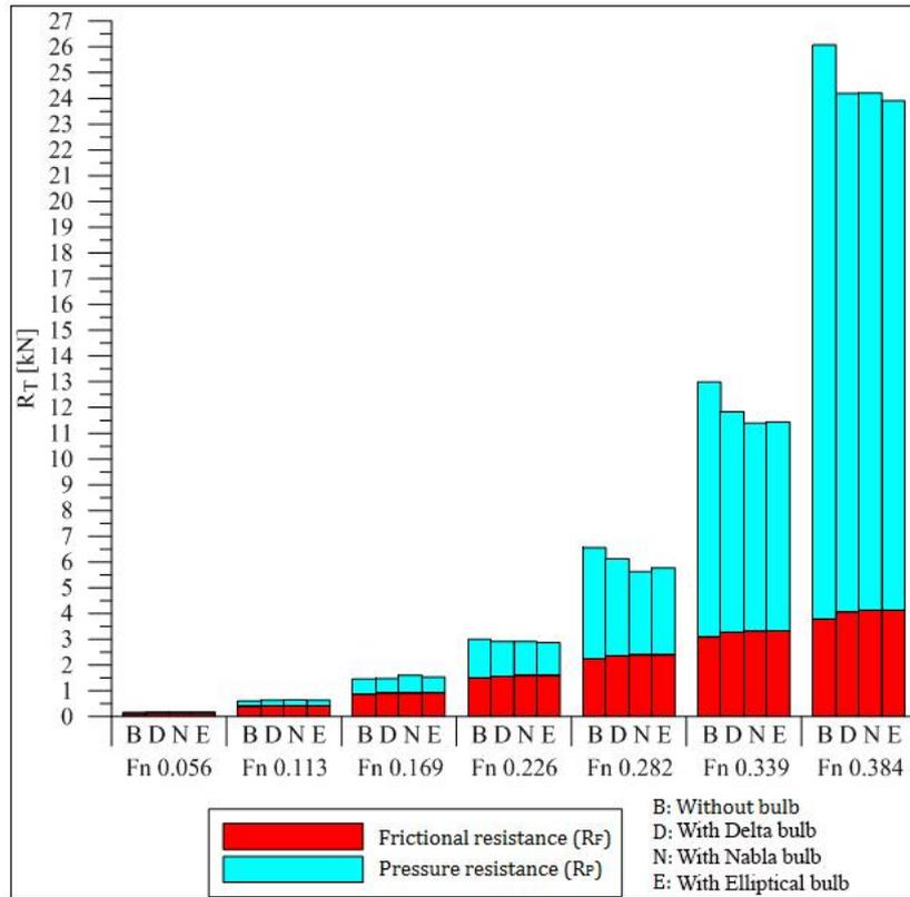
**Fig. 11** The total resistance values, which are obtained using CFD, for 148/4, 148/4-D, 148/4-N and 148/4-E coded boats
