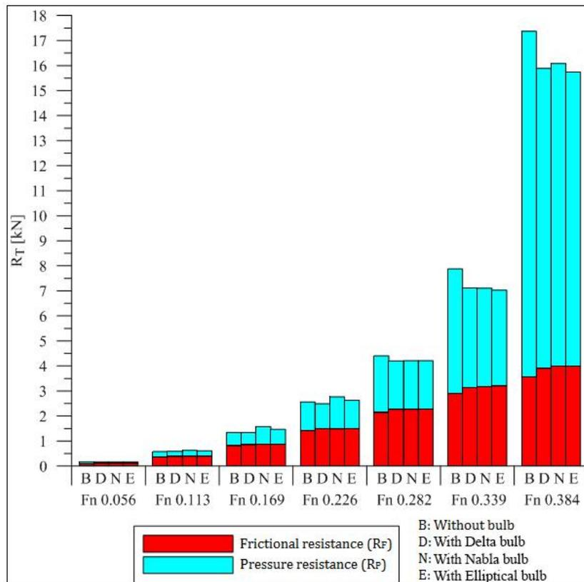
**Fig. 10** The total resistance values, which are obtained using CFD, for 148/3, 148/3-D, 148/3-N and 148/3-E coded boats
