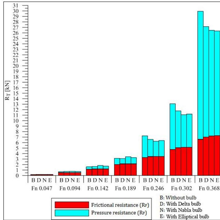
**Fig. 13** The total resistance values, which are obtained using CFD, for 148/9, 148/9-D, 148/9-N and 148/9-E coded boats
