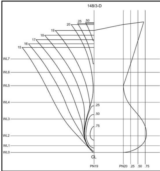
**Fig. 3** Fore cross sections plan and bulb profile of the 148/3-D code fishing boat
