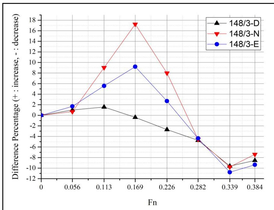
**Fig. 14** According to Fn values, increase (+) or decrease (-) percentages of the total resistance values of 148/3-D, 148/3-N and 148/3-E in reference to 148/3.
