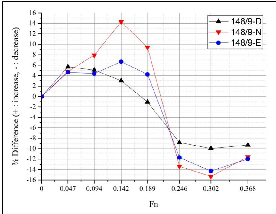
**Fig. 17** According to  $F_n$  values, increase (+) or decrease (-) percentages of the total resistance values of 148/9-D, 148/9-N and 148/9-E in reference to 148/9.
