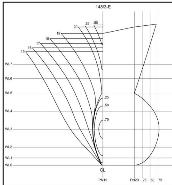
**Fig. 5** Fore cross sections plan and bulb profile of the 148/3-E code fishing boat
