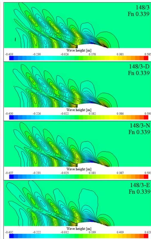
**Fig. 19** Wave deformations at the free water surface of 148/3, 148/3-D, 148/3-N and 148/3-E coded boats at  $Fn$  0.339
