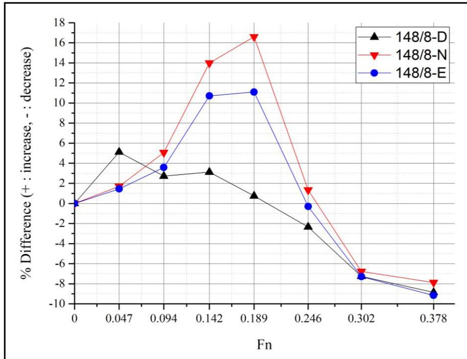
**Fig. 16** According to Fn values, increase (+) or decrease (-) percentages of the total resistance values of 148/8-D, 148/8-N and 148/8-E in reference to 148/8.
