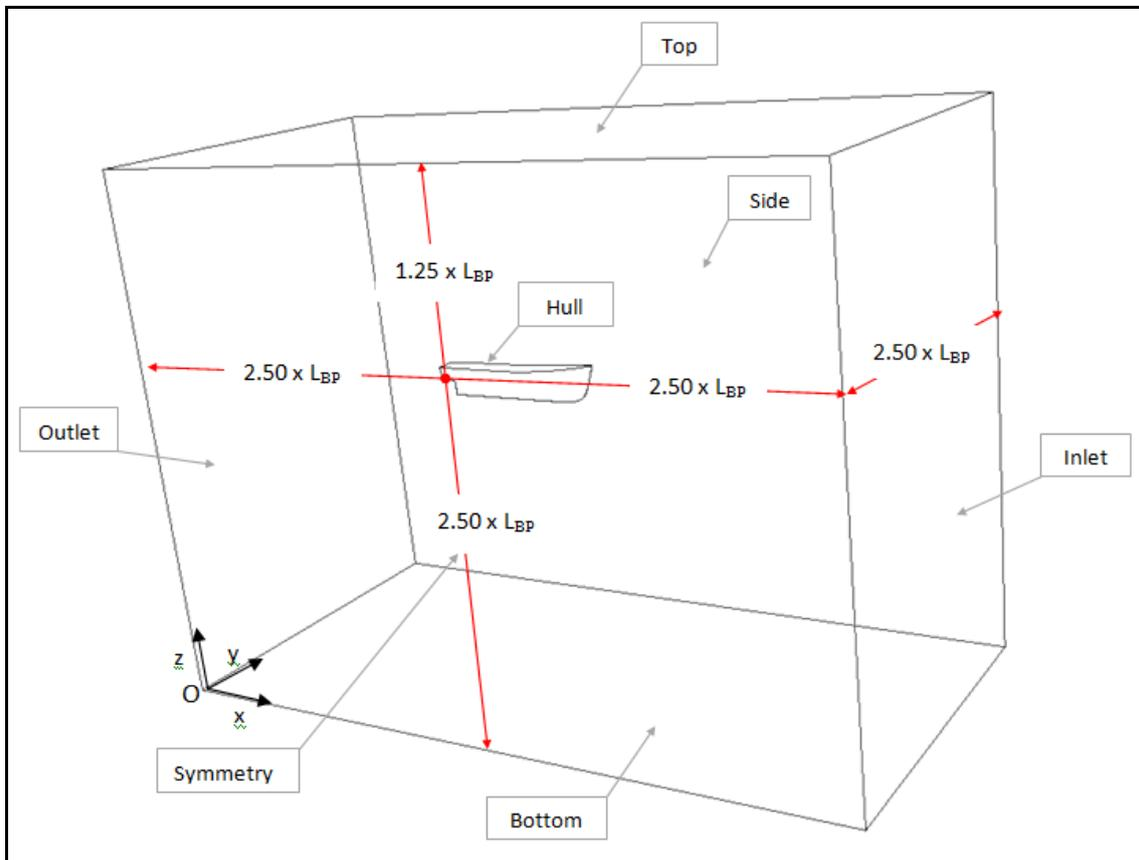
**Fig. 7** The dimensions of the computational domain and the names of the surfaces
