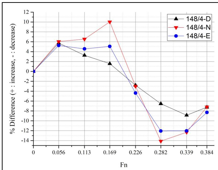
**Fig. 15** According to  $F_n$  values, increase (+) or decrease (-) percentages of the total resistance values of 148/4-D, 148/4-N and 148/4-E in reference to 148/4.
