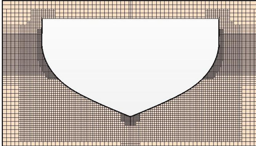
**Fig. 9** Boat cross section mesh structure
