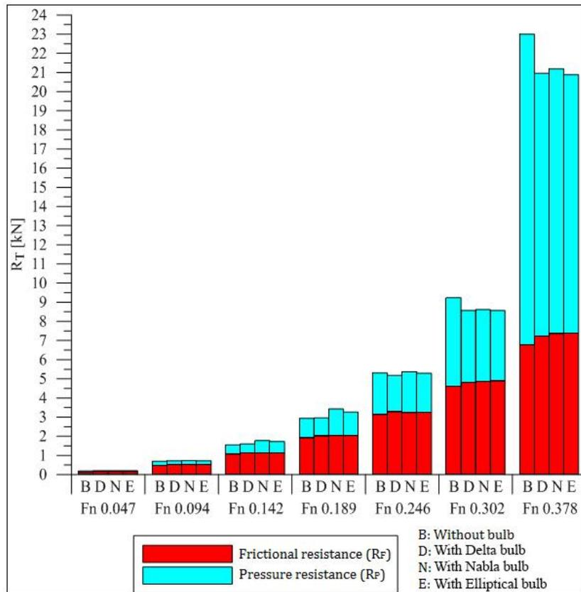
**Fig. 12** The total resistance values, which are obtained using CFD, for 148/8, 148/8-D, 148/8-N and 148/8-E coded boats
