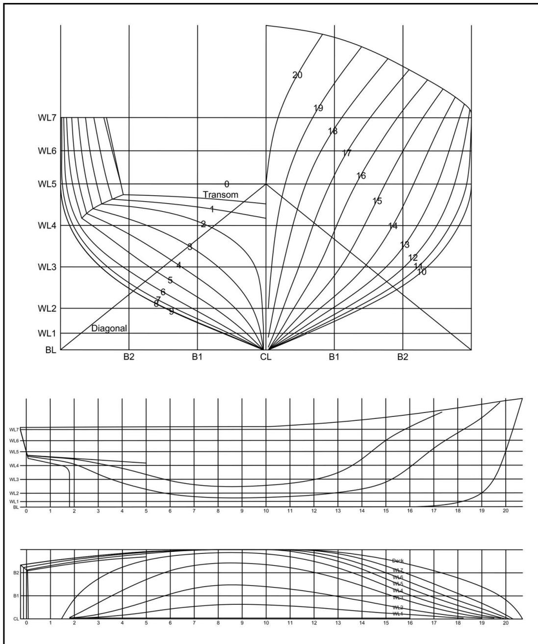
**Fig. 2** Lines plan of the 148/3 coded fishing boat [29]
