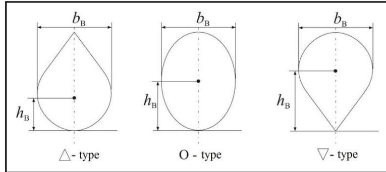
**Fig. 1** The sections of the bulbs
