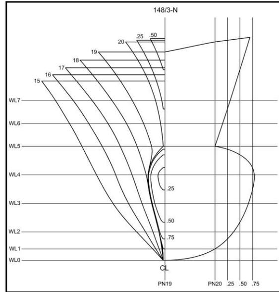
**Fig. 4** Fore cross sections plan and bulb profile of the 148/3-N code fishing boat
