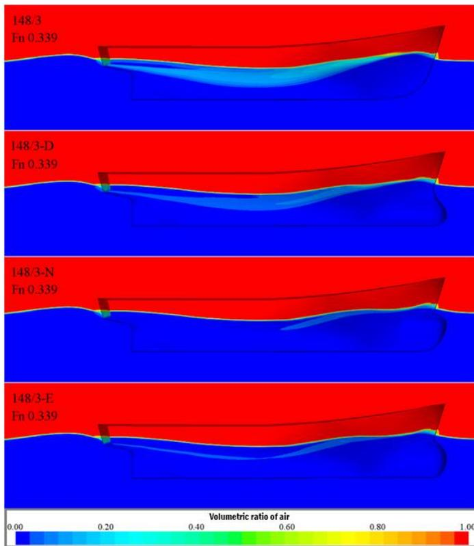
**Fig. 18** Wave deformations occurring in the boat symmetry plane of 148/3, 148/3-D, 148/3-N and 148/3-E coded boats at  $Fn$  0.339
