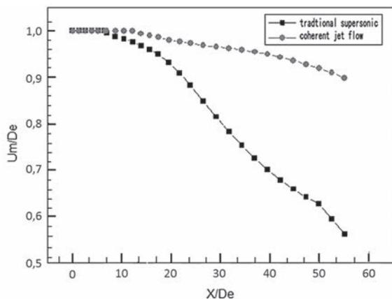
**Figure 3** Velocity attenuation of the main oxygen flow along the axis with high temperature CO<sub>2</sub> accompanying.
