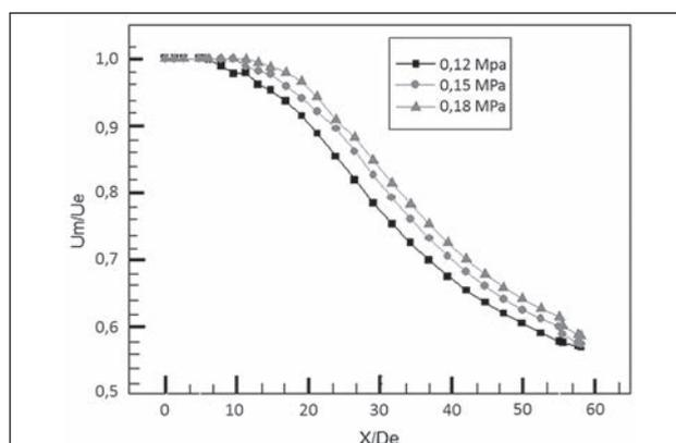
**Figure 5** Velocity attenuation of coherent jet along the axis with CO<sub>2</sub> accompanying of different pressure
