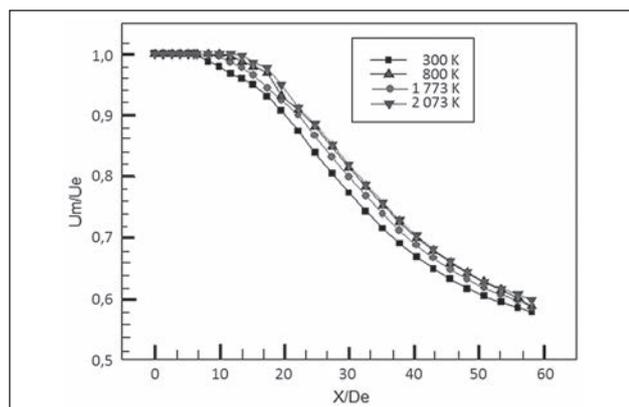
**Figure 4** Velocity attenuation of coherent jet along the axis with CO<sub>2</sub> accompanying of different temperature
