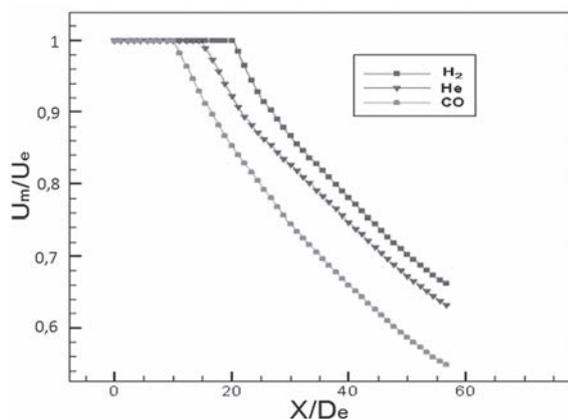
**Figure 2** Velocity attenuation of the main oxygen flow along the axis with different gas accompanying
