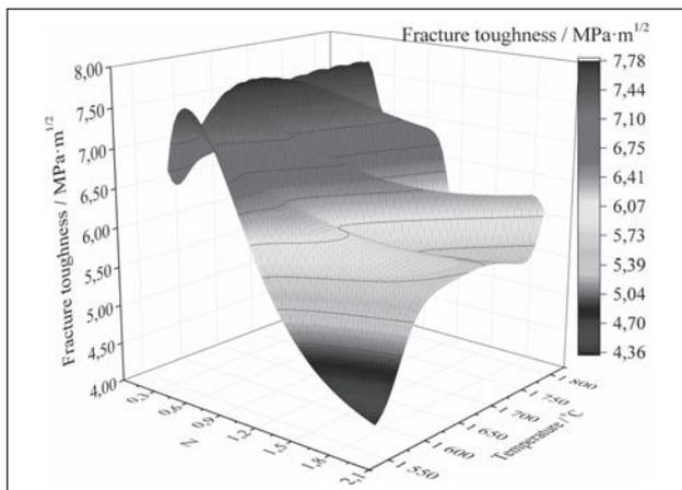
Figure 6 Fracture toughness versus Z and temperature
