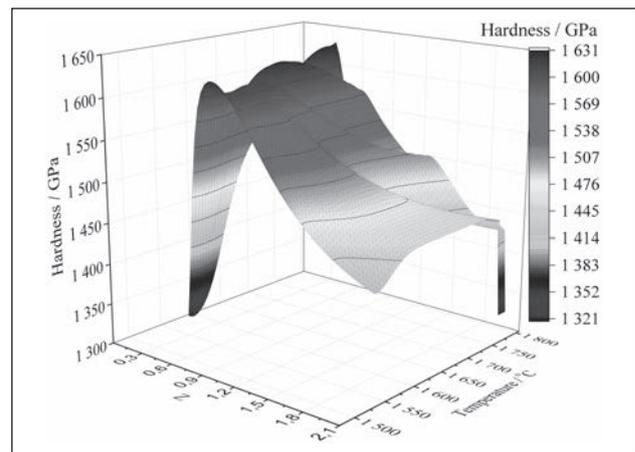
Figure 5 Hardness versus Z value and temperature
