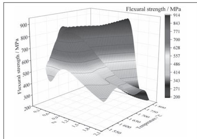
Figure 7 Flexural strength versus Z and temperature
