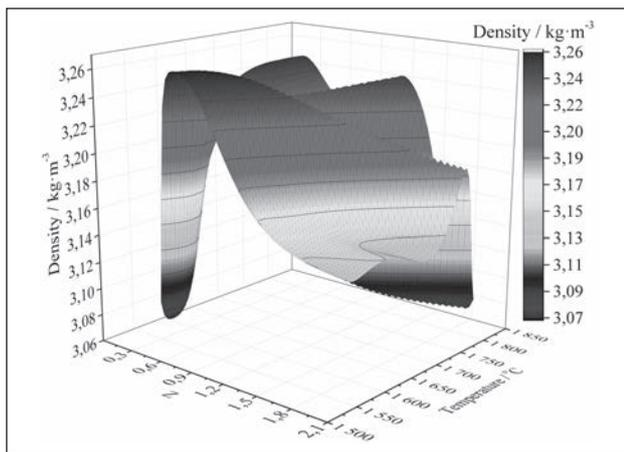
Figure 4 Bulk density versus Z value and temperature
