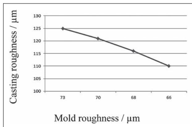
Figure 5 Dependence between the mold and the ingot surface roughness
