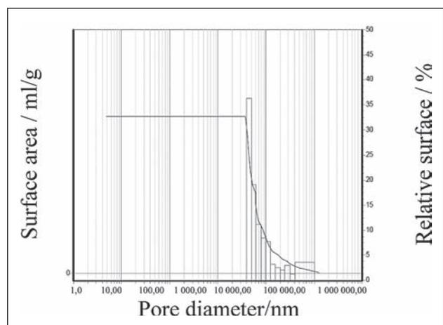
**Figure 3** Pores distribution in the SRM ingot
