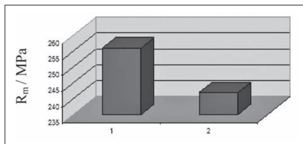
Figure 4 Histogram of tensile strength of the ingots obtained in different conditions: 1 – SRM, 2 – SCM
