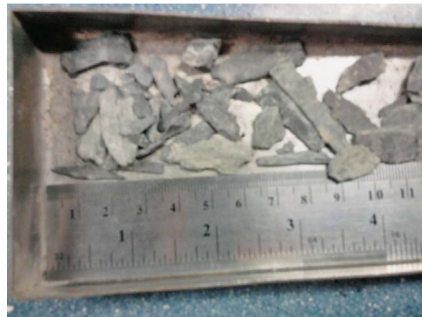
Figure 2: Rock particles cavings in shape of splinters (Zadravec, 2012)
