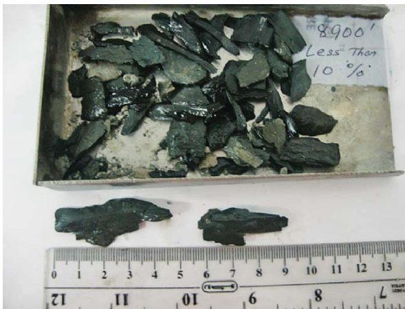
Figure 4: Rock particles cavings in shape of angulars (Zadravec, 2012)
