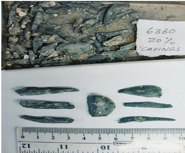
Figure 3: Rock particles cavings in shape of tubes (Zadravec, 2012)
