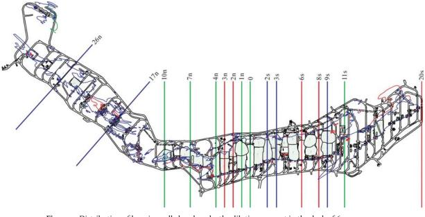
**Figure 3:** Distribution of hangingwall chambers by the dilution amount in the deck of 640 – 740 m. The amount of ore dilution in the chambers:  $\Box$  <2.0%;  $\Box$  2.0-4.0%;  $\Box$  >4.0%
