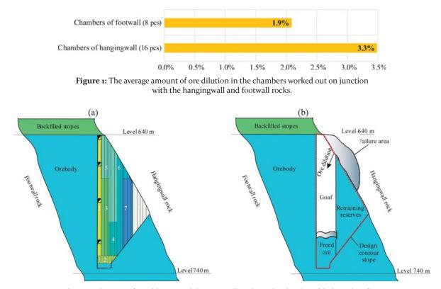
**Figure 2:** Schematic diagram of ore dilution with hangingwall rocks in the chamber: (a) the order of ore extraction in the chamber; (b) ore dilution from the chamber on junction with hangingwall; 1 – 8 numerical order
