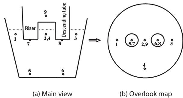
**Figure 2** Tracer add position diagram
