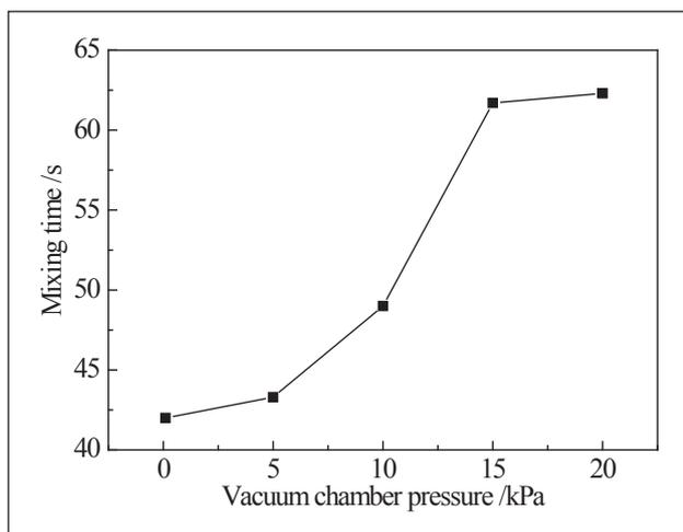
**Figure 7** Mixing time under the different pressure of the vacuum chamber
