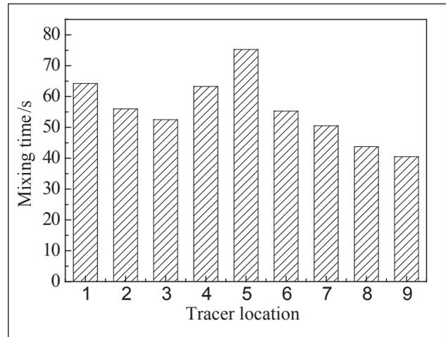
**Figure 3** Mixing time of tracer at different positions when blowing volume is 1 200 NL/min
