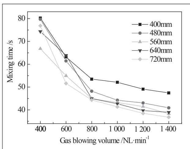
**Figure 4** Effect of blowing volume on mixing time under different immersion depths
