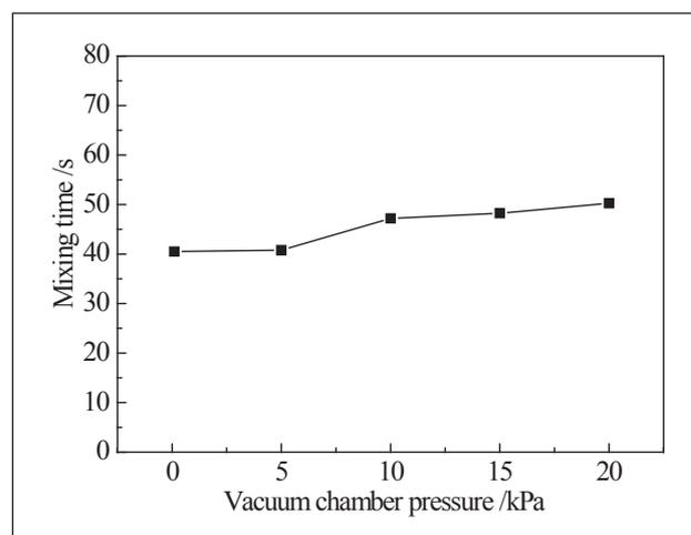
**Figure 6** Mixing time under the different pressure of the vacuum chamber
