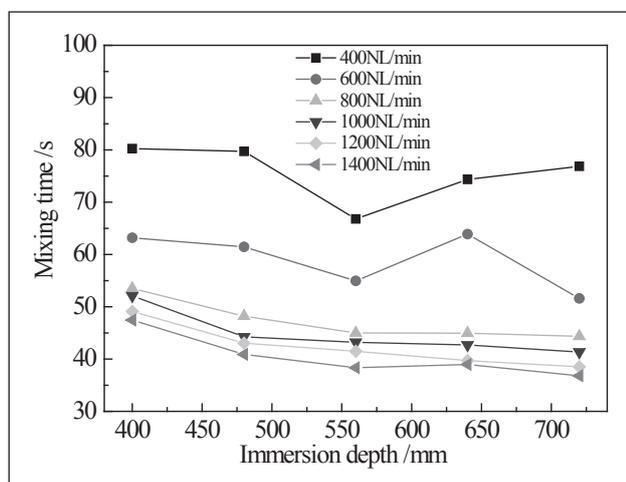
**Figure 5** Effect of immersion depth on mixing time under different blowing conditions
