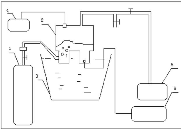
**Figure 1** 1 Air tank 2 Vacuum chamber model 3 Ladle model 4 Differential gauge 5 Vacuum pump 6 Velometer
