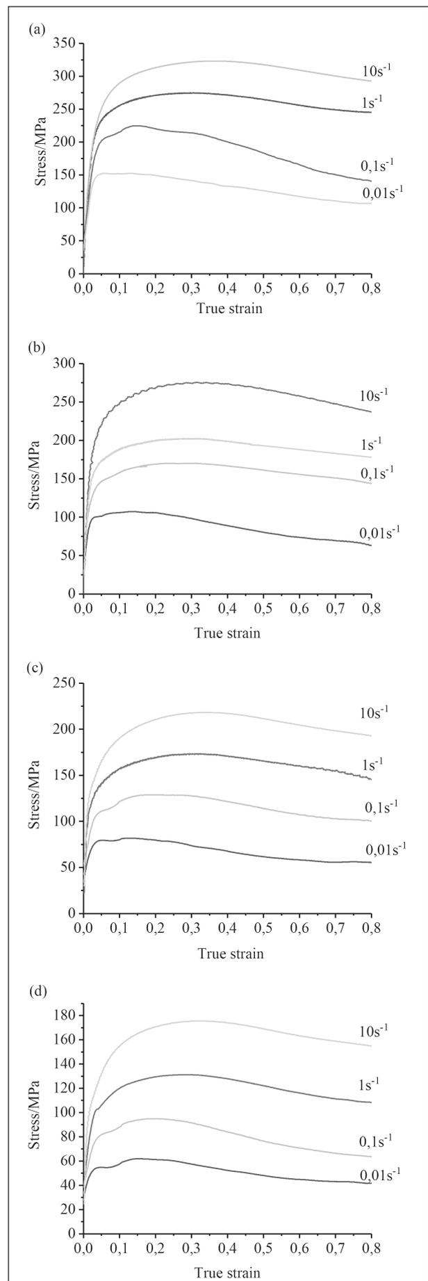
**Figure 1** True stress – strain curves of 3Cr23Ni8Mn3N obtained by hot simulation compression tests. (a)  $T = 1\ 000\ ^\circ\text{C}$ ; (b)  $T = 1\ 060\ ^\circ\text{C}$ ; (c)  $T = 1\ 120\ ^\circ\text{C}$ ; (d)  $T = 1\ 180\ ^\circ\text{C}$ .
