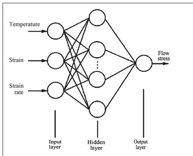
Figure 2 Schematic map of BP neural network
